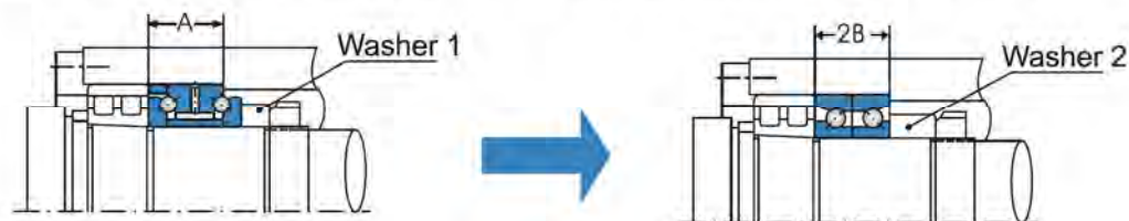
Fig. 5 The mounting of high-speed angular contact thrust ball bearings
